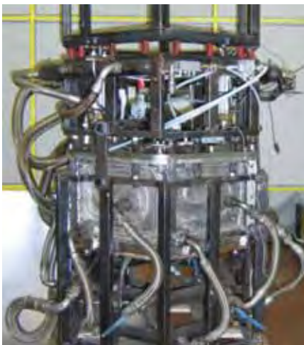
Figure 1: Mould (on left) with pipework to distribute heating and cooling fluid, and moulded part (on right).
