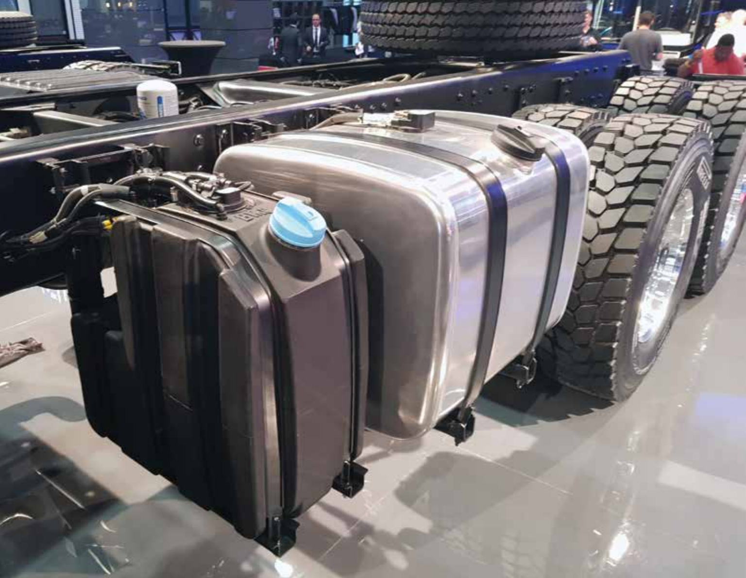
An aluminum diesel tank of a heavy commercial vehicle next to a rotomolded adblue tank.
